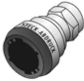
Pressure testing push-adaptor with female thread made of stainless steel 1.4401, incl. EPDM sealing components and withdrawal barriers, can be disassembled, to pressure-test Steelfix and copper pipes
