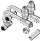
Push SL-radiator connection set made of non-porous metallized brass, suitable for processing with carbon steel, stainless steel and copper pipes, heating/cooling connection pipe d12x1mm, incl. height- and depth-adjustable corner shut-off valve, the longitudinal interference fit pipe connection of the shut-off valve is ensured with an M13 hex key at the front of the shut-off valve, locking is by means of a 4mm Allen key, radiator connections 3/4" female, flat sealing
