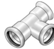
Press-tee equal or reduced made of carbon steel coated with a zinc layer, incl. EPDM sealing components, d15-54 "leak before pressed"
