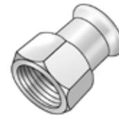
Press-adaptor with female thread made of carbon steel coated with a zinc layer, incl. EPDM sealing components, d15-54 "leak before pressed" Press contour: M
