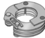
Press loop for pressing STEELFIX and COPPERFIX system components using a WZ281 press adapter d67-108/1 and d108/2mm and a WZ274N KELIT press machine (ACO 203 XL)
