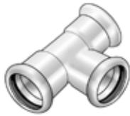
Press-tee equal or reduced made of carbon steel coated with a zinc layer, incl. EPDM sealing components, d15-54 "leak before pressed" Press contour: M
