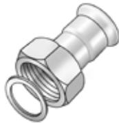
Press-fit transition screw connection with female thread for connecting to fittings, made of carbon steel coated with a zinc layer, incl. EPDM sealing components, d15-54 "leak before pressed" Press contour: M
