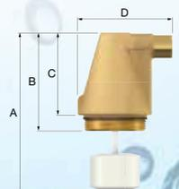
\* K<sub>v</sub> = Q / √ΔP Q: Flow [m³/h] ΔP: Pressure loss over product [bar]
