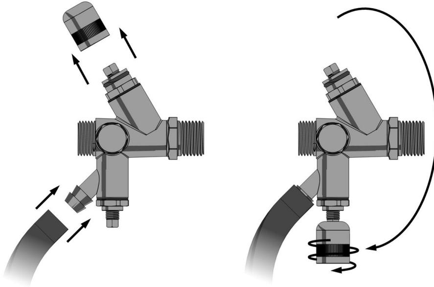
Locate the bleed screw on the pump. The following diagrams show examples of typical bleed screw locations for most pumps:
