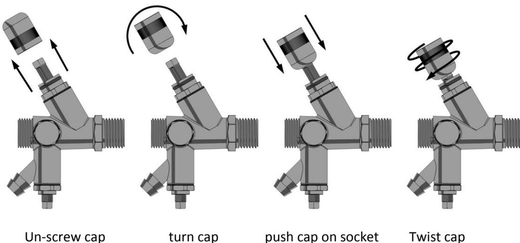
Attach a length of hose to the hose tail on the drain valve and put the other end to drain. Then, using the cap off the isolation valve, open the drain valve:
