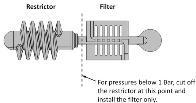
To install the flow restrictor/filter, hold it by the tab and push it into the opening of the float valve connection, as shown in the diagram below:
