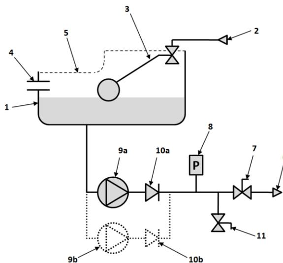
The pressurisation unit is fitted with a break tank (1) which is filled from the mains water supply (2) via a float operated valve (3). The break tank is fitted with an overflow (4) in case the break tank overfills, and a weir overflow (5) in case the primary overflow fails.
