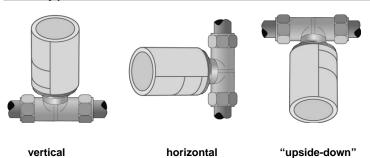
The KM596 should preferably be installed in a vertical or horizontal assembly position. With "upside-down" assembly, specific circumstances (e.g. sewage water) may reduce the service life.
