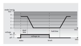
With the currentless-open version, the valve is closed evenly by the plunger movement when the operating voltage is switched on – after the dead time has elapsed.
