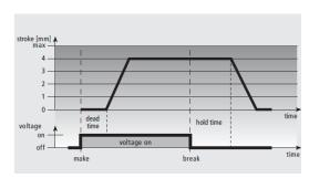
With the currentless-closed version, the valve is opened evenly by the plunger movement when the operating voltage is switched on – after the dead time has elapsed.
