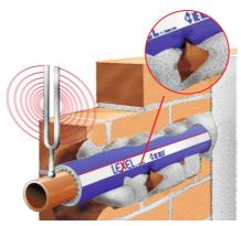
Caution! Damaged insulation or residual mortar between the pipelines, wall or floor screed can cause the formation of sound bridges, which transmit noise unhindered. In the interest of effective sound insulation, acoustic decoupling using pipe insulation should therefore be as gap-free as possible.
