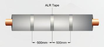
Securely tape the slit and butt joints with ALR Tape. ALR Tape should be applied in bands around the pipe with a maximum gap of 500 mm between bands.
