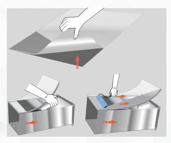
**(b)** Align the insulation edge with duct edge and gently lower the sheet exposing only required adhesive and pad firmly on the insulation as it lays on the duct from the fixed edge moving to the other edge ensuring air is expelled. Then, apply uniform pressure over the insulating material with the help of a smooth roller or with the help of hands.
