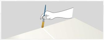
When pressed together, the material is under compression and is not stretched. Apply an additional wet seal along the butt joints.
