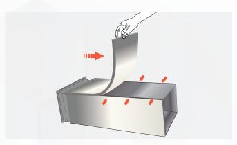
**Note:** Remember to roll the sheet down into position along the insulated edges.
