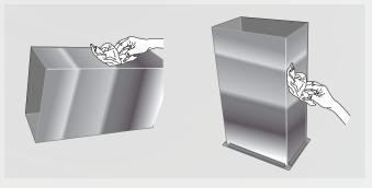
Apply FlexiCell® glue or an authorized glue by Hira Industries Technical Department. Application should be according to this installation manual on the insulating material and the flat surface.
