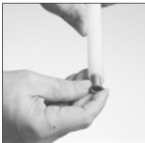
Assemble the swivel nut, cutting ring and ball valve.
