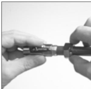
Tighten the swivel nut with your fingers and then with a wrench by the number of turns indicated in the table on the next page.
