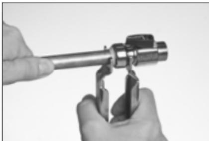
Check both the tube and the fitting for any damage before re-establishing the joint.
