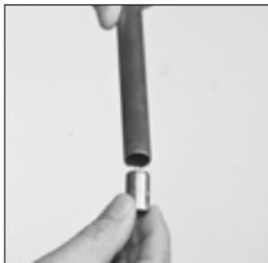
Fit the swivel nut, cutting ring and fitting.
