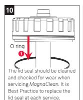
Only use Silicon grease or water to lubricate O ring. **Do not use flux or EP grease.**
