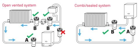
Note: In both diagrams, position A is best practice, Position B is suitable if space is tight on the return.
