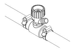
3 Remove the RapidFlush lever valve and tri-clamp fitting from the box. Add PTFE sealing tape to the thread before tightening. Ensure washer provided is fitted between tri-clamp and lever arm. Do not over-tighten. Attach to one end of the hose with the jubilee clip provided.
