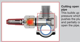
Cutting open the pipe This builds up gas pressure which pushes the plunger and partially cuts
