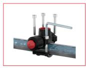
Attach the T-plus to the pipe and secure with four bolts. Models from 11/2" are supplied with click-in nuts; the bolt is clicked in, then screwed into place.
