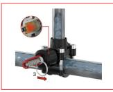
Pull the pin (3). This makes a clean cut in the pipe, creating the branch. And that's all there is to it!
