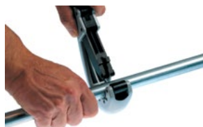
Fig. 3: Cutting the Pipe
