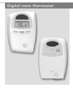
Digital room thermostat with infrared transmission, (incl. PTC-electric heating element) for room temperature control using the Design radiators. The infrared transmitter has a clear LCD display, simultaneously showing the room temperature, target temperature, operationmode and the BOOST symbol.
