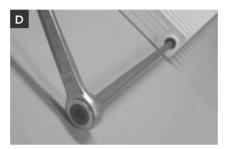
Guide the nipple turning key through a port of the last block that was fixed up to the nipple. The square drive of the nipple turning key is provided for the purpose of using the ratchet.
