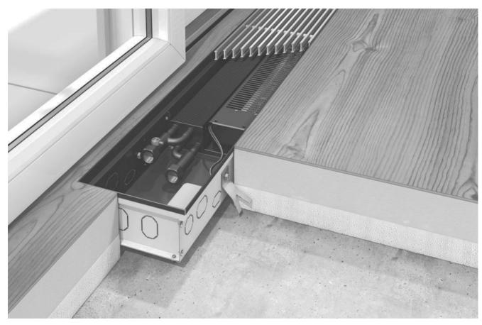
The Intratherm F1P Trench convectors succeed the original series of FPT convectors with fans. They offer a cost-effective variant with increased heat output, reduced noise level and minimal operating costs. The length of the fan has been chosen in such a way that the largest possible area of the heat exchanger is supplied with air. The heat output of the convector can be controlled either by hot water or by the air from the fan. All fans are fitted with energy-saving 12 V EC motors.
