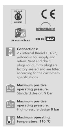
$Guarantee \ statements \ are \ available \ to \ download \ at \ {\bf www.vogelundnoot.com/download}$ panels are also delivered with factorysealed drain plugs and pivotable vent plugs. (Exception: bottom-oppositeend connection models come with a dummy plug instead of the drain plug.) Standard design: rectangular steel pipes, 70 x 11 x 1.5 mm
