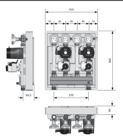
External dimensions of the thermal insulation:
