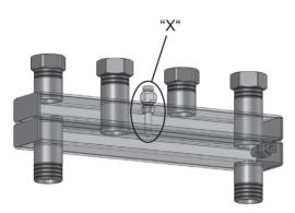
For low differential pressure installation: Disassemble valve and reassemble rotated by 180°.
